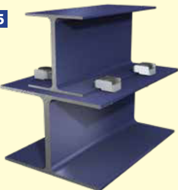
Drilled I-Section running parallel to another I-Section
