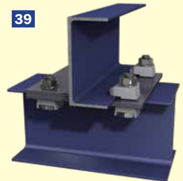
Channel positioned above I-Section at 90 degrees
