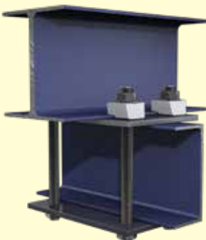
Channel section below I-Section at 90 degrees
