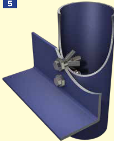
Angle to vertical hollow section post
