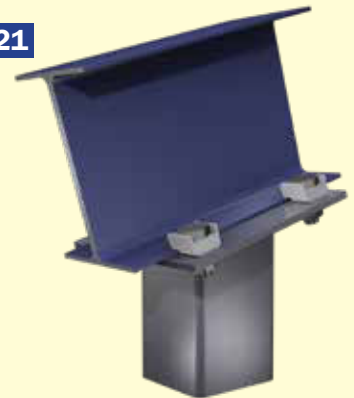
Column end plate to sloping I-Section
