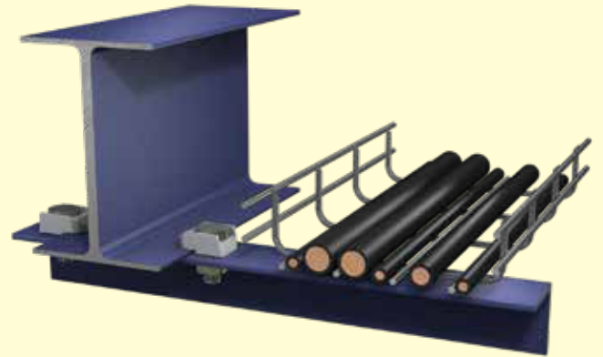
Cantilevered angle support for running cable tray
