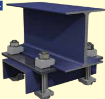
Channel section at 90 degrees below an I-Section
