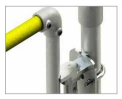
**1.** Open up gate assembly and fit U bolts, washers and nuts. Align fixing plate, ensuring top rail of gate is level with guardrail.
