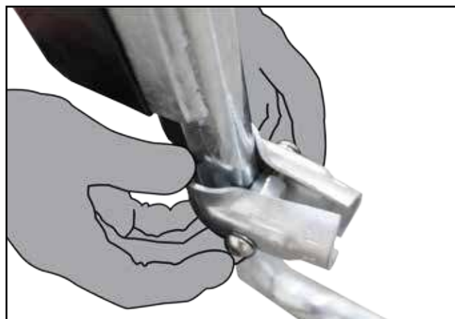
O. Mount clamp on lower part of gate, just above the bend and insert mid rail. Use 6mm hex head socket to tighten supplied M10 bolts into coupling nut.
