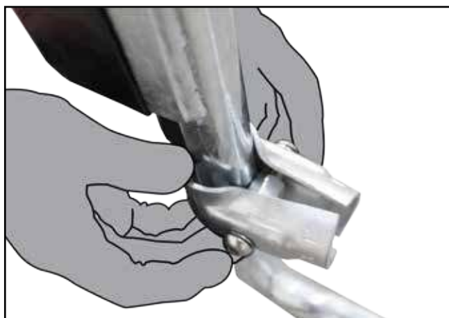
P. Mount clamp on lower part of gate, just above the bend and insert mid rail. Use 6mm hex head socket to tighten supplied M10 bolts into coupling nut.
