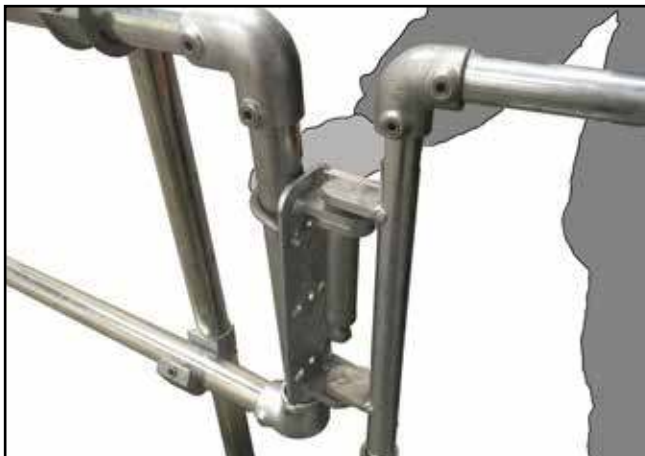
A. Align the fixing plate on internal face of the opening, so that the rails of the Safety Gate match up with the top of the Guardrail System. Select the correct U Bolt & pass around the support leg/structure and feed through the top holes of the fixing plate.
